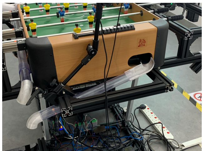
Figure 6. 3D-printed part for the exit at the side of Table Football.
