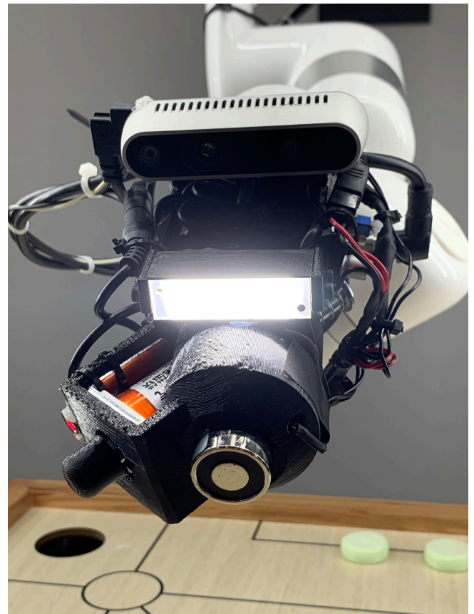
Figure 2. 3D-printed part attached around the head of the robot arm.
